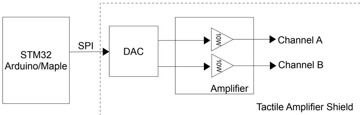
*Illustration 1: Tactile Shield Block Diagram*
